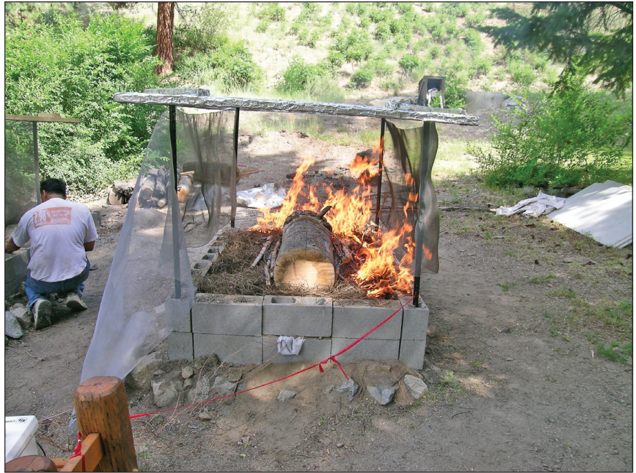
Researchers test how log size and state of decay affect soil heating. They found that rotten logs burned longer than the sound logs, leading to high soil temperatures and deeper soil heating.
