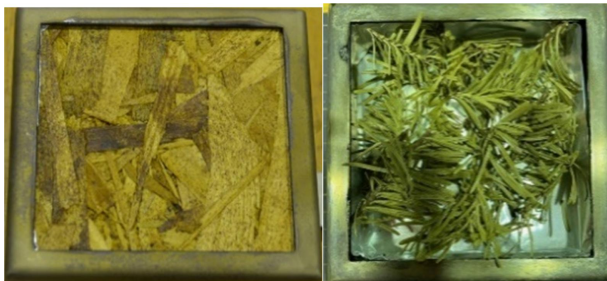
Fig. 4. OSB sample is shown on the left and noble-fir branch samples are shown on the right.
