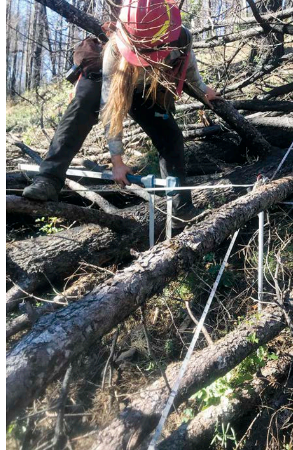
Sarah Harrison is measuring woody fuel loadings along a transect in a plot on the Mendocino National Forest. Photo by Morris Johnson, USDA Forest Service.
